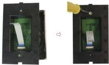
4. Cover touch panel Look at the direction of touch panel, install the ribbon cable and then cover the touch panel
