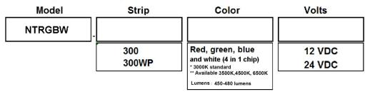
The strip must be connected to a low voltage output power supply according to selected voltage and power criteria WP indicates a weatherproof strip inside a flexible silicone sleeve.
